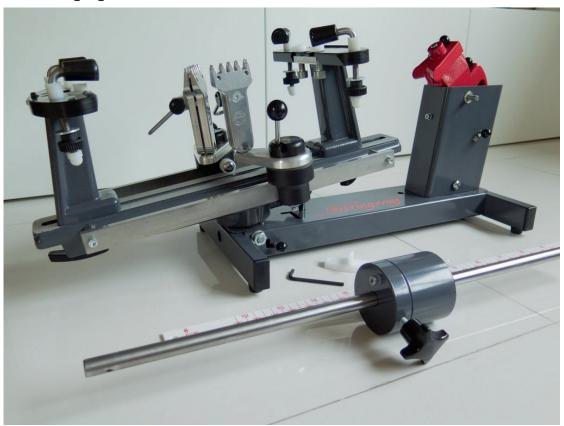
Our stringing machine (Stringway ML100-T92 with Concorde system) is one of the most accurate machines on the market with a true constant pull drop weight tensioning system. Every stringing job is also done using Stringway Cross Stringing tool which helps avoid notching, damage to the strings, while keeping profiled poly-base strings from twisting while weaving.
